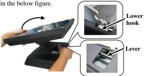
4.2 Tilt the screen up or down to your desired angle. Please do not press on the LCD panel while setting up the tilt angle.
