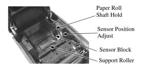
are a plastic thumb for bobbin size adjustment and a sensor block in the wall. Adjust the thumb to change the proper position of sensor block. For desktop application, the sensor block should be above the bobbin seating of paper compartment when paper near end. The acceptable paper roll bobbin outer diameter is between 18 and 24 mm.
